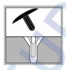
1. Tighten screw until flush with the work-surface.
