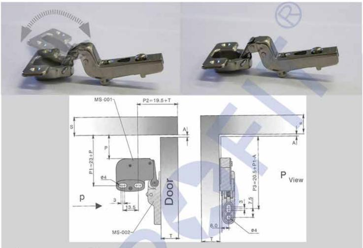
S....top panel thickness T....door thickness
