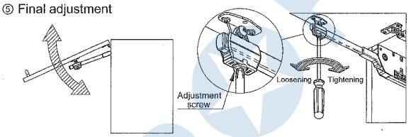
· If you feel that the door is too light (self lift-up) or too heavy (self-closing), it is possible to limit the action of the spring by tightening the adjustment screw.
