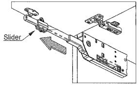
·Line up the Slider with the pin of the mounting plate
