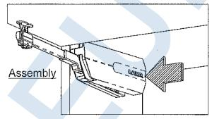
Fix the front of the cover and then clip the back in place.
