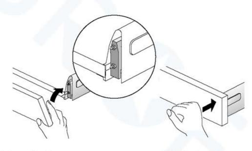
Insert hole marking jig in drawer profile Align front panel and mark drilling positions
