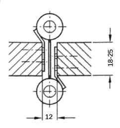
> Features: For flush timber frames 180° swing action on both sides.
